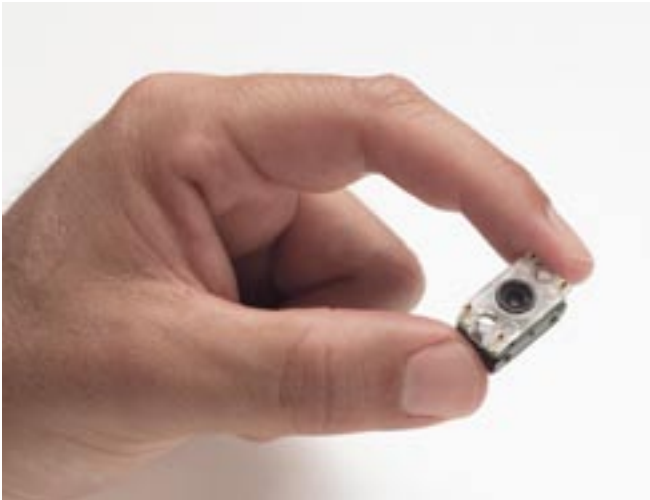
Figure 4 – Hand Held Products IT4000 and IT5000 Mini Engine Series is a critical Adaptus Imaging Technology building block. Implementing a CMOS camera, it is the eyes of the Adaptus Imaging Technology platform.
